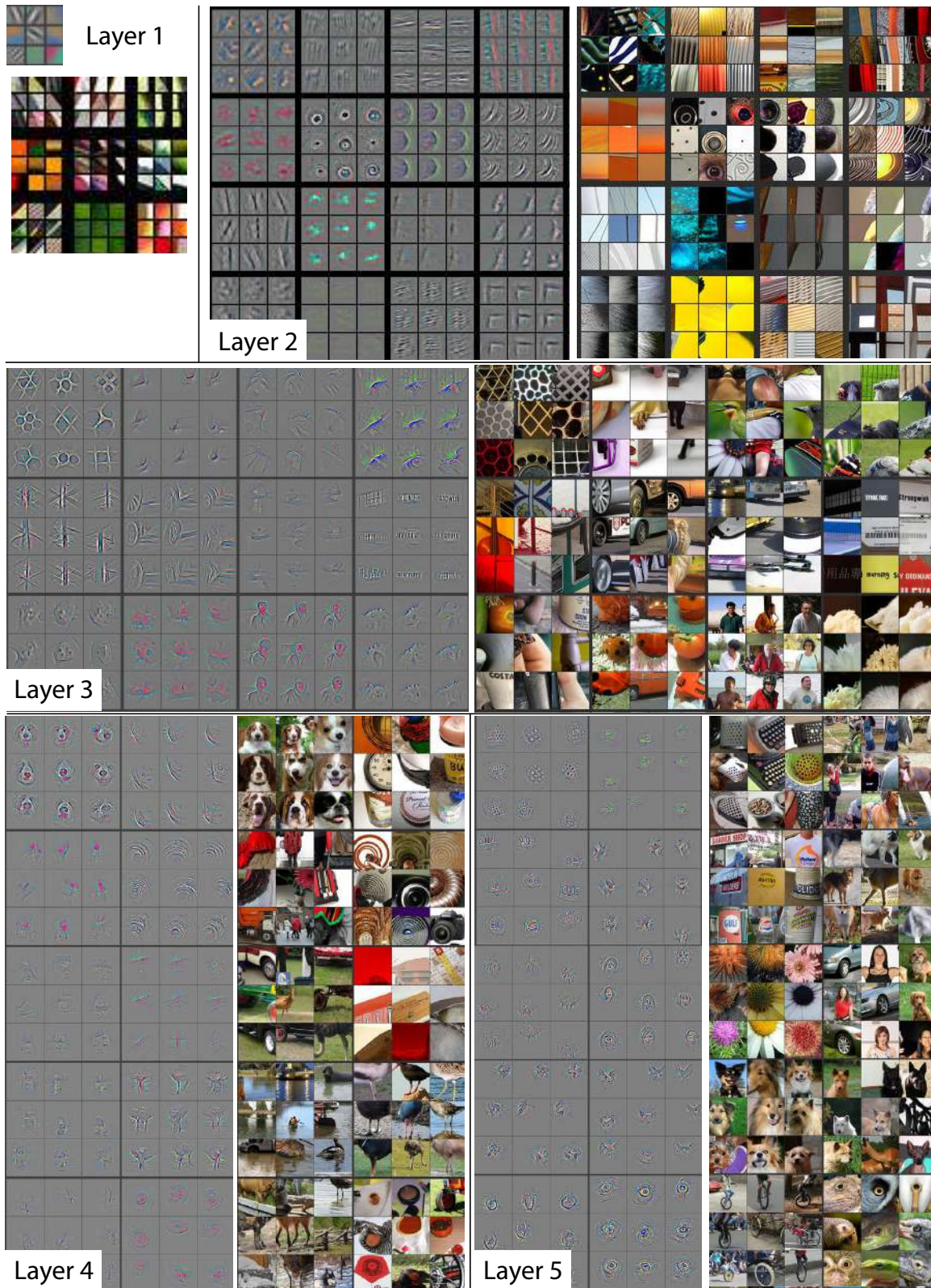
Figure 2. Visualization of features in a fully trained model. For layers 2-5 we show the top 9 activations in a random subset of feature maps across the validation data, projected down to pixel space using our deconvolutional network approach. Our reconstructions are not samples from the model: they are reconstructed patterns from the validation set that cause high activations in a given feature map. For each feature map we also show the corresponding image patches. Note: (i) the the strong grouping within each feature map, (ii) greater invariance at higher layers and (iii) exaggeration of discriminative parts of the image, e.g. eyes and noses of dogs (layer 4, row 1, cols 1). Best viewed in electronic form.
